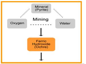
Figure 1: Mine Water Process
